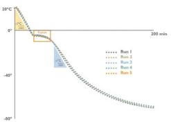
Performance test: A temperature probe was placed into a 2.0 mL cryogenic vial containing 1.0 mL of water and the tube was inserted into a room temperature CoolCell®. The CoolCell was placed into a -80°C freezer and the temperature rate and profile was recorded over a 3 hour period. The test was repeated 5 consecutive times. Conclusion: CoolCell generated identical fusion time and cooling profiles over five consecutive freeze cycles.
